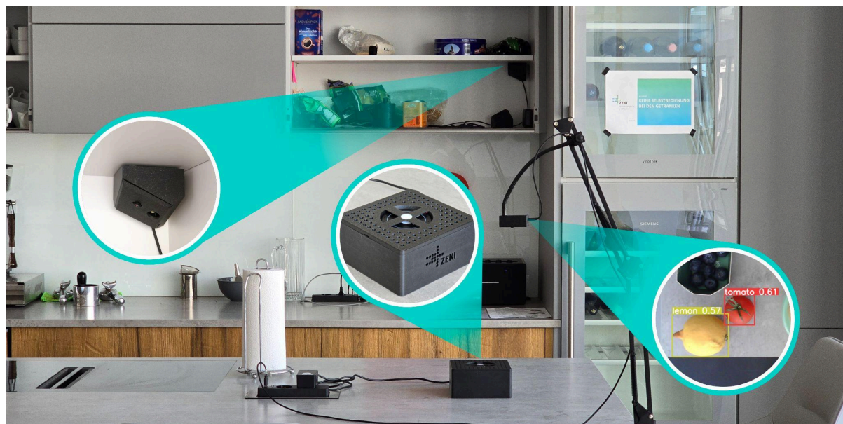
FIGURE: The Smart Kitchen setup showing ESP-32 camera placements and item recognition using YOLOv8-Worldv2.
