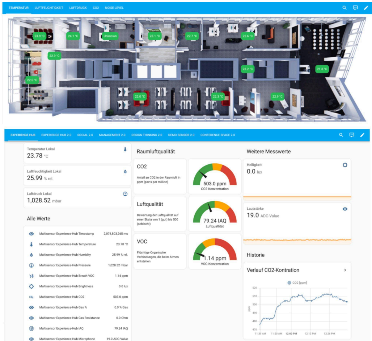
FIGURE: Visualization dashboard: Overlay of environmental metrics on the ZEKI floor plan using Home Assistant.
